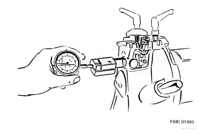
Operate fuel-injection pump at setting-point speed and measure delivery.
